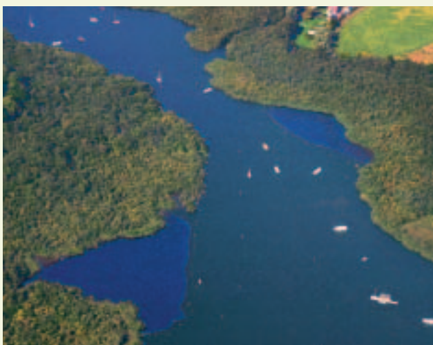
A major project has been completed at Barton that included dredging the entire broad to improve water quality and increase water depth for navigation. The latest initiative to install fish-proof barriers has proved effective in creating clear water conditions (seen here as darker areas of water).
