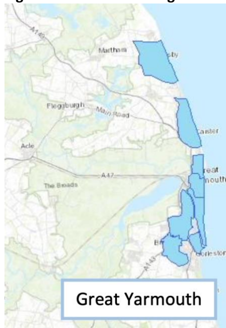
Figure 21: Critical Drainage Catchments in Great Yarmouth
