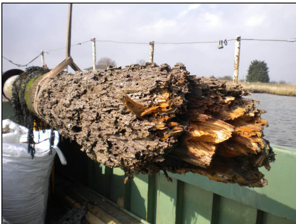
Photo 1: Broken navigation marker with significant gribble worm attack.
