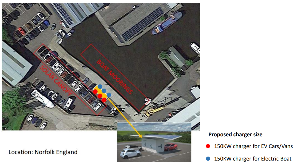
Figure A5.5: Boatyard solar augmented dual purpose EV/MEV charging station
