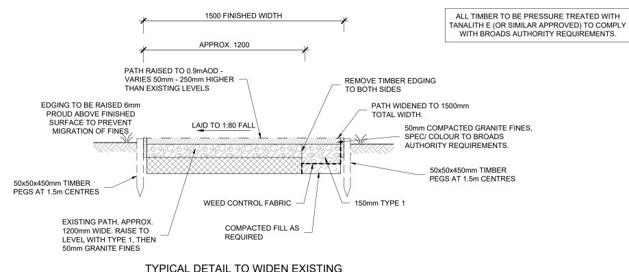
TYPICAL DETAIL TO WIDEN EXISTING FOOTPATH, LEVEL RAISED
