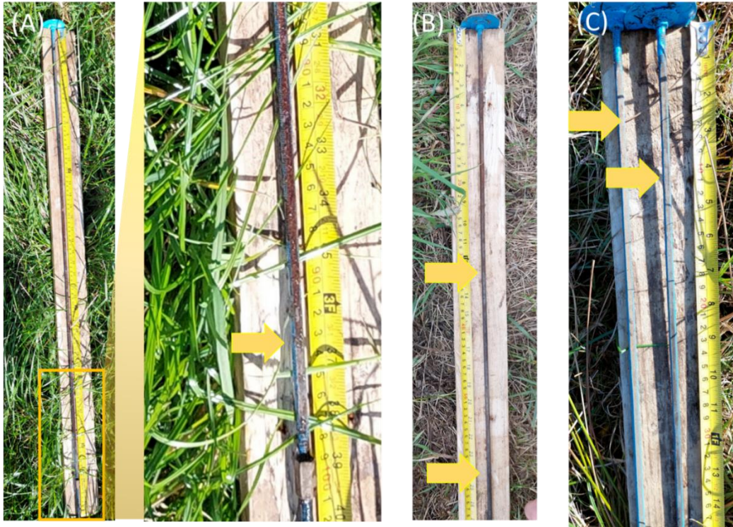
Figure 1 (A) Point of measurement of orange rust (iron oxide); (B) Point of measurement for orange rust (iron oxide) and lower black (reduced iron) deposits; (C) Replicated points of measurement at Leist's Farm.
