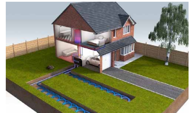
Figure 98: Example of a ground source heating system.
